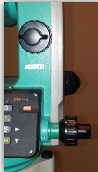
Figure 6- Fine Motion Screws
